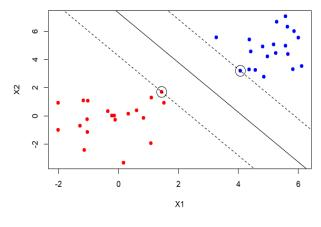
Figure 2. Diagrammatic representation of the support vectors
