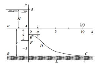
Figure 1. Flow pattern calculated at  $\epsilon=0.6,\,h_c=0.5,\,T=7,\,S=3,$  and H=5
