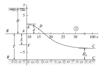
Figure 3. Flow pattern calculated at  $\epsilon = 0.6$ , T = 7, S = 3, H = 7, H<sub>0</sub> = 3, and x<sub>C</sub> = 100.
